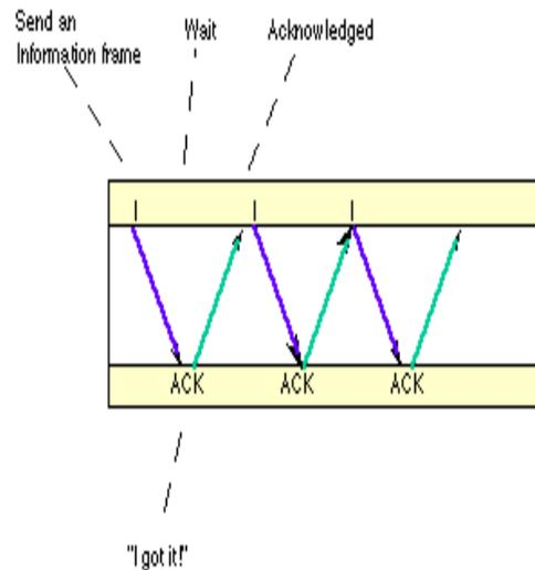
Stop and Wait ARQ - Waiting for Acknowledgment (ACK) from the remote node.
